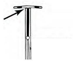
Figure C-1 Vertical Stem of T fully inside Insertion Tube
